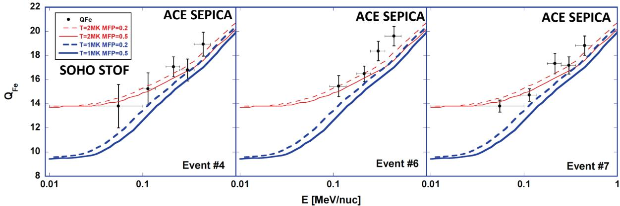
Mean Fe charge states for three impulsive energetic particle events as a function of energy together with model curves, including acceleration, stripping, and adiabatic cooling for source temperatures of 1 MK (blue) and 2 MK (red), and transport mean free paths  $\lambda = 0.5$  AU (solid) and  $\lambda = 0.2$  AU (dashed) (Kartavykh et al., ApJ, 671, 947, 2007). Typical coronal temperatures as derived from ionic charge states in the solar wind are about 1 MK ([ACE News #146](#)).
