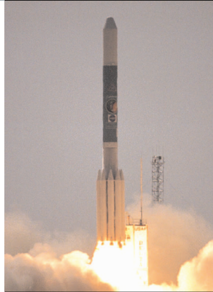
ACE was launched on a Delta II rocket in August 1997 from the Kennedy Space Center in Florida. Delta II is an expendable two-stage, liquid-fueled rocket that stands at a height of 38 m (126 ft) and weighs 232,000 kg (511,000 lb). It is currently the world's most reliable launch vehicle.
