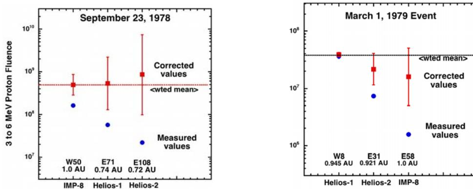
**Figure 2.** A comparison of the fluence of 3 to 6 MeV protons measured by Helios-1 & 2 and IMP-8 for the 9/23/78 and 3/1/79 events (based on measurements by Reames et al. [5]). The locations of the three spacecraft relative to the flare site are indicated. Once corrected for latitude and radius, the three estimates are in reasonable agreement.
