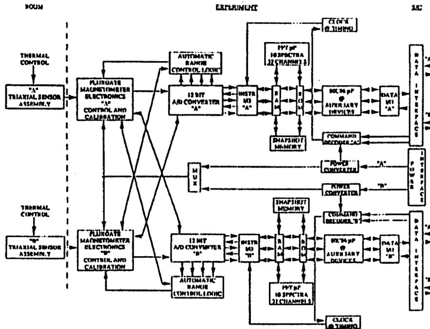
Figure 7.1.8-2: MAG -- Schematic of Standard Fluxgate Operation
