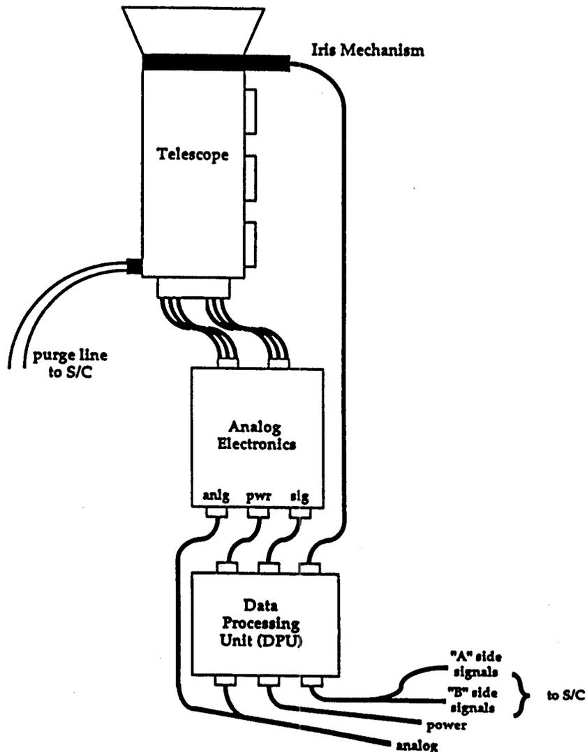
Figure 7.1.3-3: ULEIS Three Wedge Prototype Instrument
