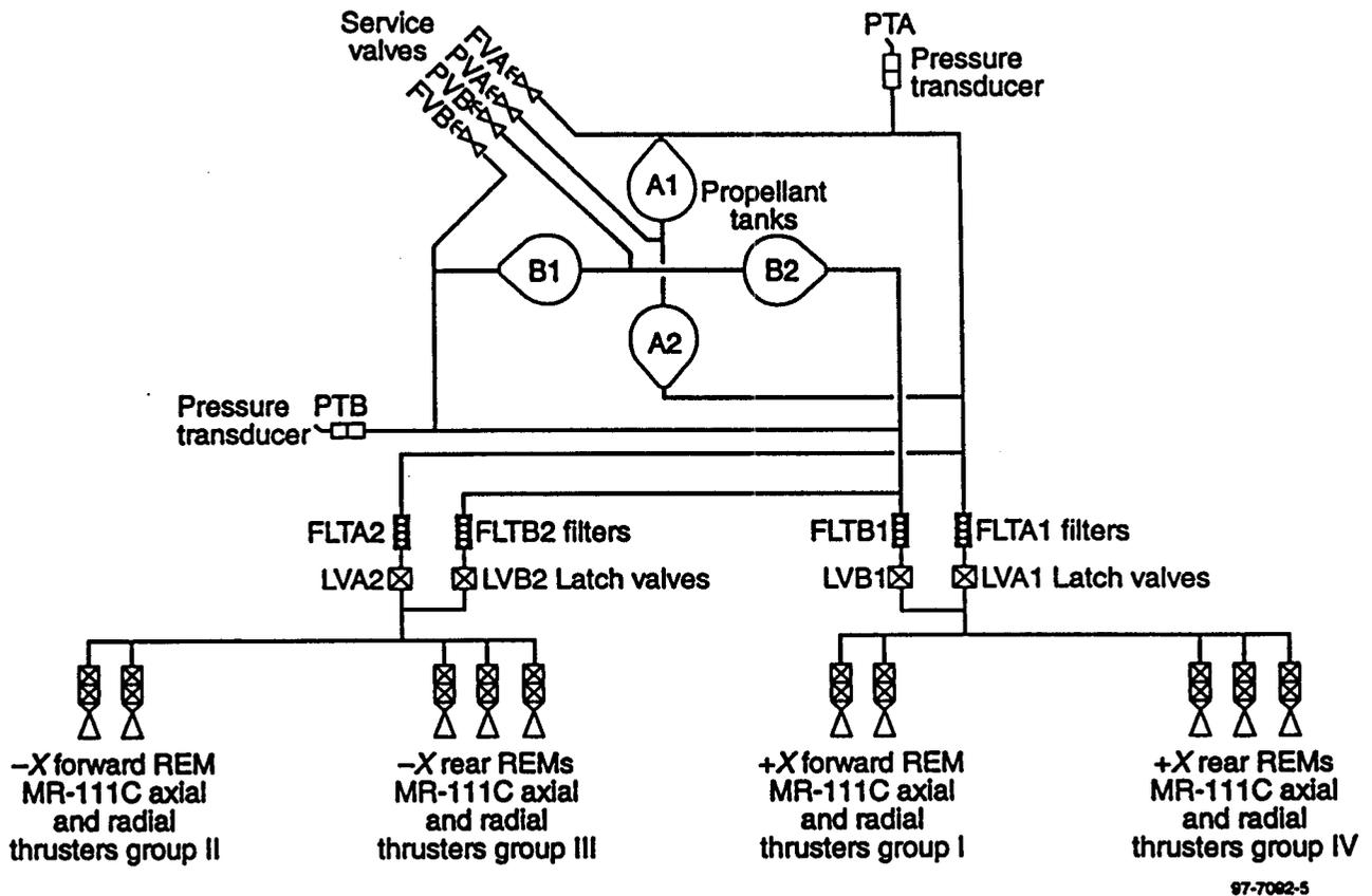
Figure 7.2.6-2: Propulsion -- Location and Function of Thrusters
