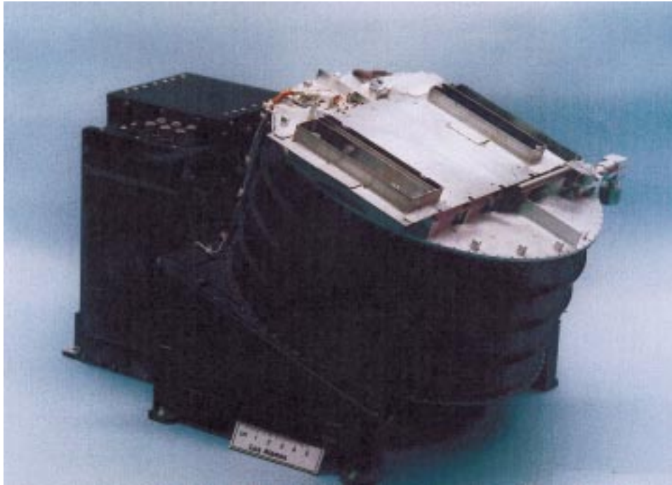
Figure 11. Photograph of the SWEPAM-I instrument. The large cylindrical housing is the sensor head; the rectangular electronics box behind it houses the high and low voltage power supplies and control electronics.
